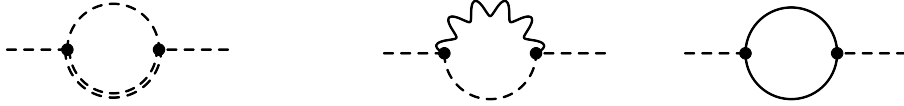
Figure 3. Higgs wave function renormalisation effects. Left: heavy-light contribution to Z_H^{(1)} in (3.8). Right: gauge-boson and fermionic contributions to the anomalous dimensions of the SSM parameters A and \kappa in (B.3) and (B.4). The wiggly line corresponds to a B_\mu or W_\mu^a field, the solid straight lines represent fermion fields, while the rest of the line styles and their meanings are identical to those employed in Figure 1.
