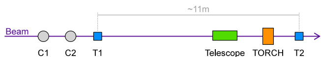
Fig. 3. A schematic showing the beam-line configuration. C1 and C2 are Cherenkov counters. T1 and T2 are timing stations spaced approximately 11 m apart.
