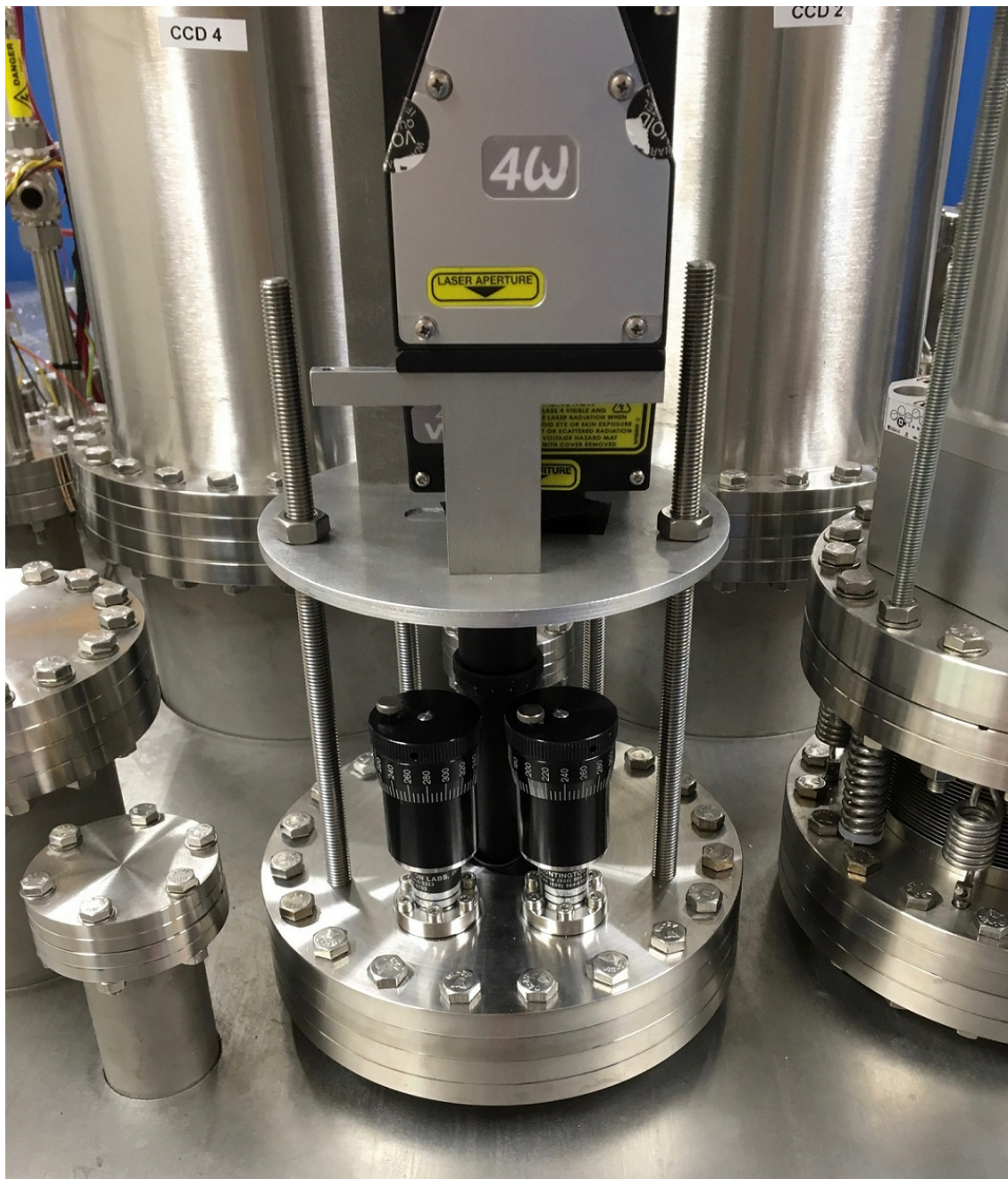
Figure 21: The Quantel Q-Smart 100 pulsed Nd:YAG laser, mounted on the top flange of the ARIADNE cryostat. Two rotary feedthroughs are used to control the position and orientation of the UV mirror.
