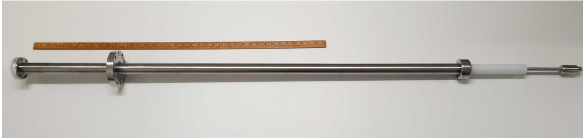
Figure 9: The ARIADNE high voltage feedthrough. A metrestick is shown for scale.
