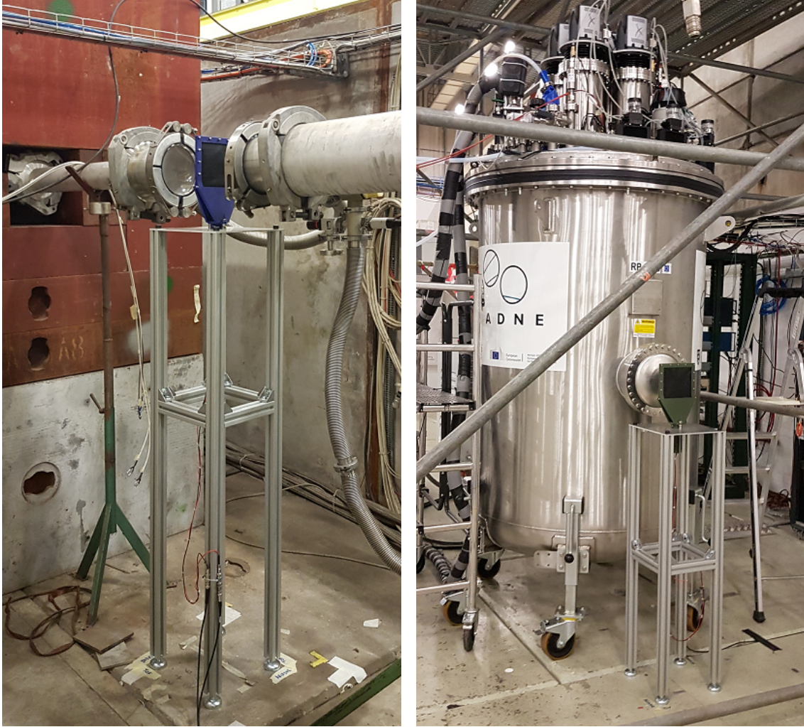
Figure 34: The far (left) and near (right) Time of Flight assemblies. The far assembly was positioned in the beamline air gap, and the near assembly directly in front of the detector's beam window. The separation between the assemblies was 18.05 m.
