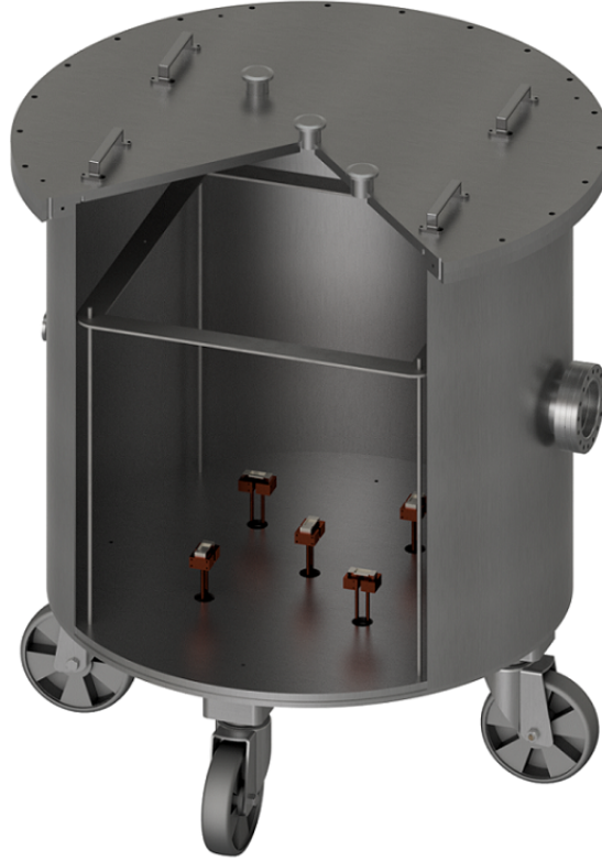
Figure 14: A CAD model of the vacuum evaporation chamber, which was used to apply a TPB coating to the PMTs, the glass plate and the reflector panels. The five crucibles for holding the TPB powder can be seen at the bottom of the chamber, along with their associated copper blocks for heating and the frame for suspending the component(s) to be coated. The viewport is shown on the right of the chamber.
