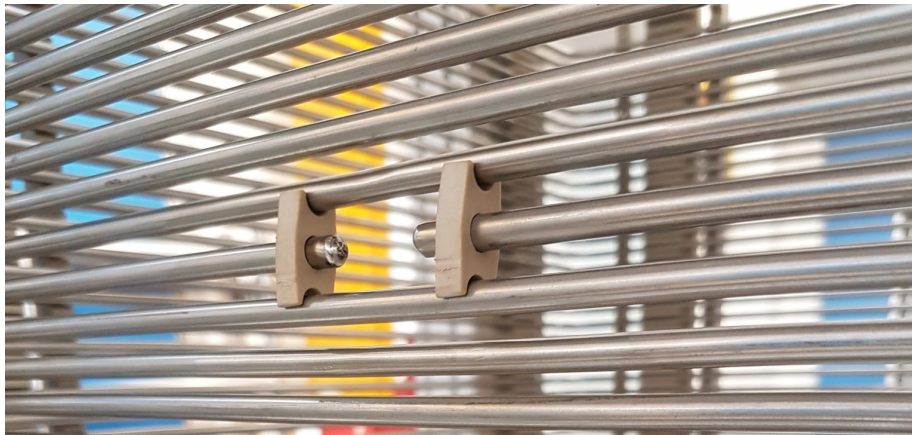
Figure 23: One of the eight small-width gaps in the TPC. The smoothed and polished ends of the field-shaping ring are supported by PEEK elements.
