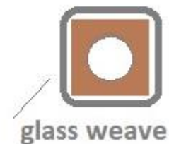
Figure 44: Profiles of hollow copper conductor and insulation (Luvata of Finland)
