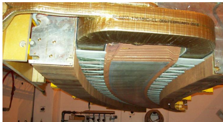
Figure 41: Dipole coil embedded in flux return yoke, seen from below
