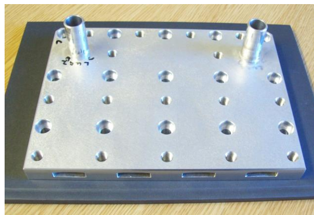
Figure 40: Aluminium heat exchanger with embedded channels seen in cross section, unit is friction-welded
