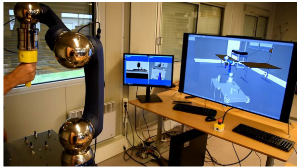
(b) An operator using the master-slave interaction system to operate a simulated robot in the Gazebo simulator.
