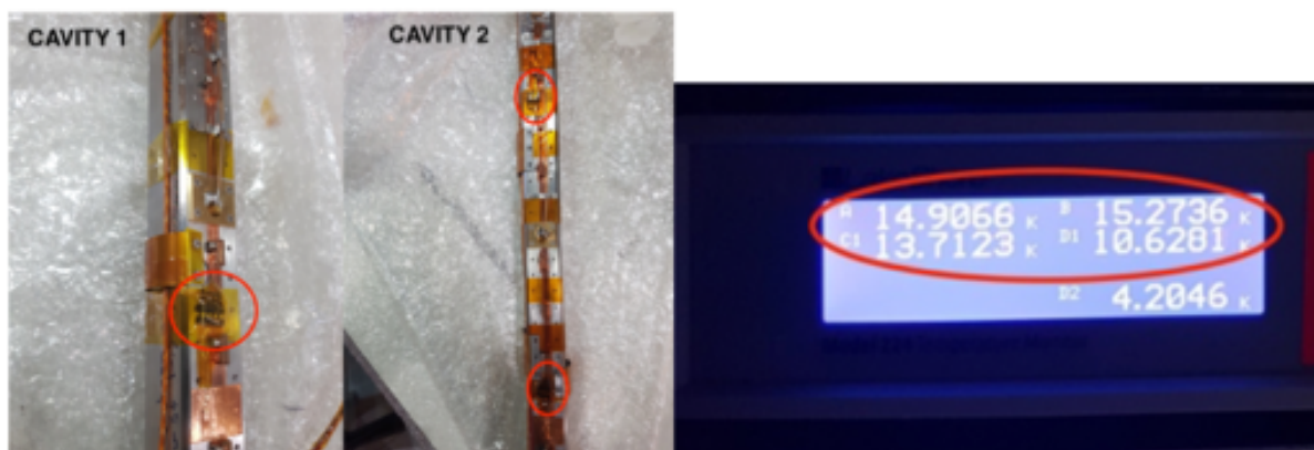
Figure 5: 1 Temperature Sensor in the middle of cavity #1 (Left) and 2 Temperature Sensors on the front and back side of cavity #2 (Middle). Screen on Lakeshore T-Monitor showing that all 4 T-sensors are working (Right).
