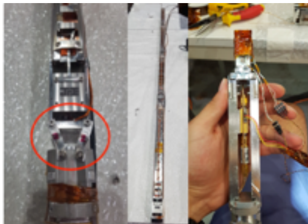
Figure 10: The metal-sheet parts that were created and installed to connect the 4 cavities together (Left) and all the 4 connected cavities before they were installed in the magnet (Middle). The “vacuum vessel” whose all electronic and RF components have been removed and has been inserted and locked on the back side of the cavities inside the magnet bore (Right).
