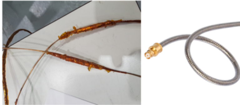
Figure 6: Old 0.047in RF cables with intermediate connectors (Left) and new 0.047in RF malleable/sucoform continuous cables (Right).
