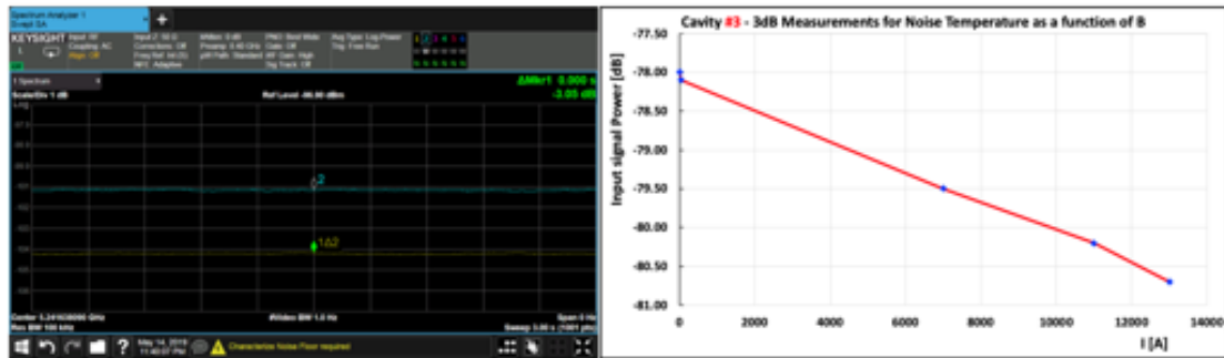
Figure 15: An example measurement for the maximum 13kA magnet current with an input of -80.7dBm (Left) and the plot with the various measurements for different currents (Right).
