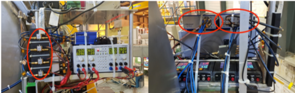
Figure 12: External pre-amplifiers (Left) and the 2 new RF Switches connected to the input and output of the cavities (Right).
