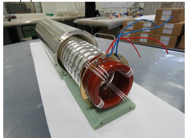
Figure 1: Trigger transformer partially out of housing and before moulding.
