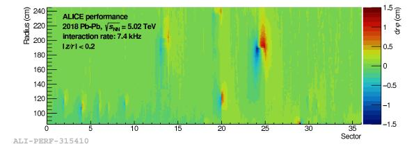
**Figure 3:** The space-charge distortions  $dr\varphi$  (color) as a function of the radius and the TPC sector for |z/r| < 0.2 in 2018 Pb–Pb data at an interaction rate of 7.4 kHz. Modified voltage settings are used in the IROCs and the OROC of sector 24 to mitigate the space-charge distortions.
