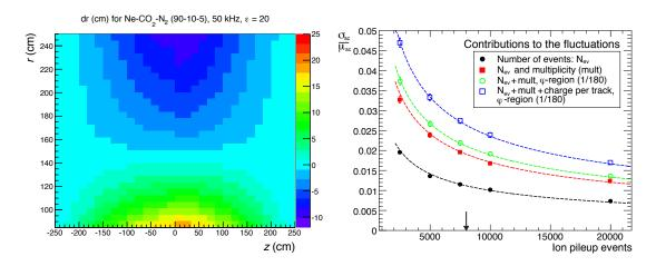
**Figure 4:** Left: Radial space-charge distortions dr (color) as a function of the radius r and the z position, expected for  $\varepsilon = 20$  in Pb–Pb collisions at 50 kHz. Right: Different contributions to the space-charge density fluctuations at 50 kHz Pb–Pb collisions from equation 3.1 (dashed lines) and toy Monte-Carlo simulations (markers).
