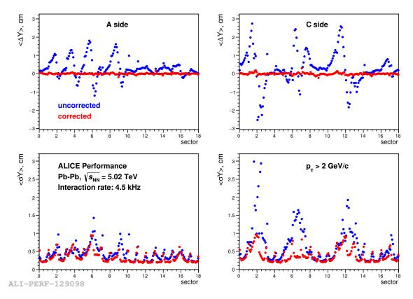
**Figure 2:** The track residuals to the vertex (top row) and the resolution (bottom row) are shown as a function of the TPC sector on the A (left) and C (right) side for uncorrected (blue) and corrected (red) data taken during the Pb–Pb period in 2015.
