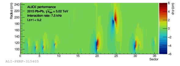
**Figure 1:** The measured space-charge distortions  $dr\varphi$  (color) as a function of the radius and the TPC sector coordinate for |z/r| < 0.2 in 2015 Pb–Pb data at an interaction rate of 7.5 kHz.
