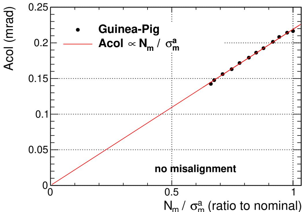
**Figure 14.** The acollinearity variable  $Acol$  predicted by Guinea-Pig simulations at each step of the ramp-up, as a function of the average bunch intensity divided by the average bunch length to the power 0.72, for leading-order Bhabha events. The result of a fit of an affine function is shown as the full line.
