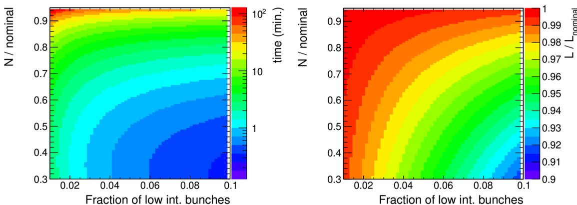
**Figure 16.** Left: Time needed to measure  $Acol_{\text{beam}}$  with a relative uncertainty of 5% in a setup with a given fraction (shown on the  $x$  axis) of pilot bunches with a lower than nominal intensity (shown on the  $y$  axis). The values of  $Acol$  predicted for leading-order Bhabha events have been used. Right: Fraction of the nominal luminosity that is kept in such a setup.
