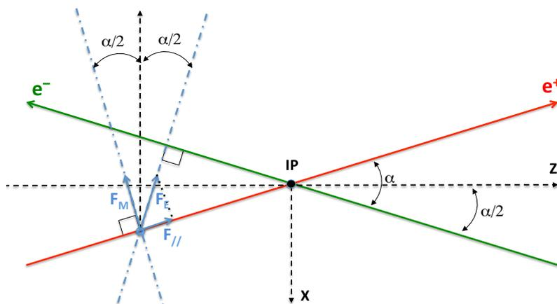
**Figure 2.** Schematic view of the electric and magnetic attractive Lorentz forces  $\vec{F}_E$  and  $\vec{F}_M$  acting on each positron from the opposite electron bunch, upon bunch crossing at the interaction point (IP). Similar forces from the positron bunch affect each electron. From ref. [15].
