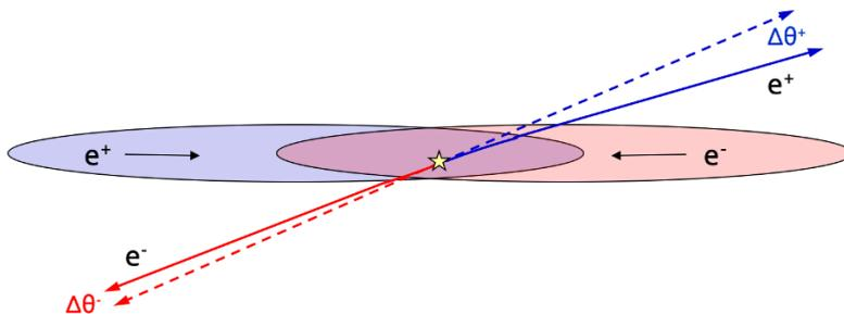
**Figure 1.** Illustration of the focusing electromagnetic force that is experienced by the charged leptons emerging from a Bhabha interaction, in the case of head-on collisions. The dashed lines show the original direction of the leptons, while the full lines show their direction after the electromagnetic deflection induced by the opposite charge bunch. The case of collisions with a nonzero crossing angle is illustrated in section 3.3.
