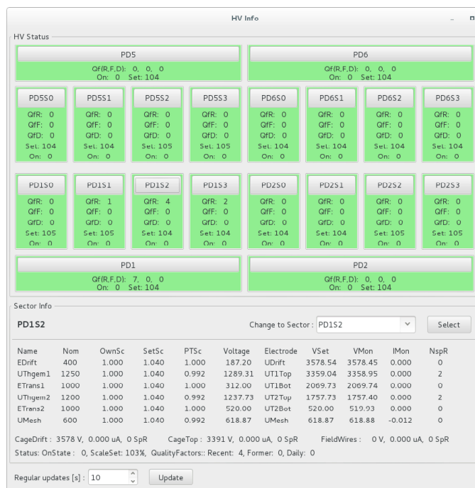
Figure 12: Screen shot of the main frame of the graphical interface, providing information on all the detector sectors, the spark counts, and details of the selected PD1S2 sector.
