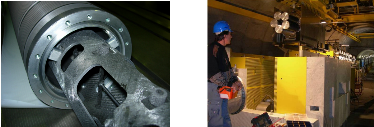
Figure 4.6: The CNGS target. Left: detail of a target head with the graphite rods the support structure and the external aluminium cylinder. Right: photo during the installation of the target unit with the five heads in its place in the beam. The side iron and marble shielding and the forced-air duct at the bottom are visible. In the final installation a top shielding with remotely movable blocks is installed.
