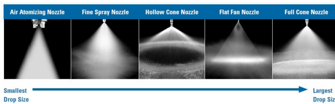
Figure 4.48: Industrial nozzles used for cooling of metal castings.
