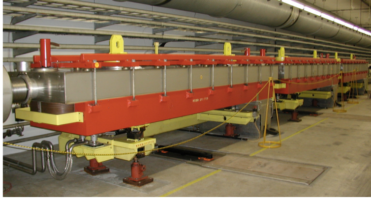
Figure 3.11: Existing MSSB splitter magnets at the top of TT20, which would need to be replaced by a new bipolar laminated design.
