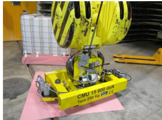
Figure 6.30: 3D drawing (left) and photo (right) of the electrical double twist lock hook used for the handling of shielding blocks.
