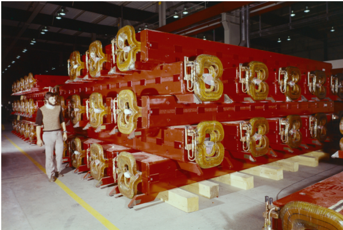
Figure 16: SPS Main Dipole Magnets in storage before installation [25].
