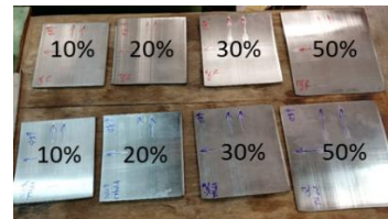
Figure 4: Eight sub-sheets cross-rolled to 10 %, 20 %, 30 % and 50 % nominal thickness reduction respectively. The sheets from the top were eventually submitted to the HT at 650°C for 24h.
