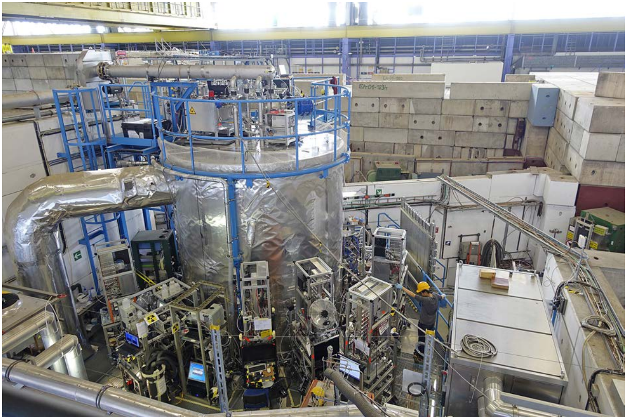
Fig. 1: CLOUD in the East Hall T11 beam line of the CERN Proton Synchrotron, during the CLOUD13 run, September-November 2018. The stainless-steel chamber (3.0 m diameter, 26 m 3 volume) is located inside a thermal housing around which air circulates at a temperature between 208 K and 313 K, with a stability near 0.01 K (the air return duct can be seen to the left of the thermal housing). The chamber is surrounded by an array of state-of-the-art instruments that continuously sample and analyse the contents of the chamber. Five different lights sources for the chamber mimic sunlight by targeting specific photochemical reactions. A 3.5 GeV/c \pi^+ beam of about 1.5 m transverse dimension provides controlled ionisation rates over the full range occurring in the troposphere. The beam emerges from the green dipole magnet at the right-hand edge of the image and passes through an x - y counter hodoscope before crossing the chamber. Neutral (ion-free) conditions are simulated with a high-voltage clearing field, which sweeps ions from the chamber in under 1 s. The chamber is supplied with synthetic air from the evaporation of liquid nitrogen and liquid oxygen. The air is humidified with ultrapure water, and ozone is added from a UV generator. A flexible, ultra-clean and highly-stable gas system supplies the chamber with up to around 25 trace gases at concentrations as low as 1 pptv (part per trillion by volume) from concentrated sources that include gas bottles, evaporators and generators. Two stainless-steel fans at the top and bottom of the chamber, respectively, ensure the contents of the chamber are well-mixed. In order to maintain cleanliness inside the chamber, the fans are magnetically coupled to external drive shafts and motors. For ‘CLOUDy’ experiments, the chamber is operated in a classical Wilson cloud chamber mode by performing controlled adiabatic pressure reductions of a humid air parcel. This maintains a liquid or ice cloud in the chamber for 5-10 minutes, to allow investigation of direct ion-aerosol-cloud interactions and other cloud microphysical processes.
