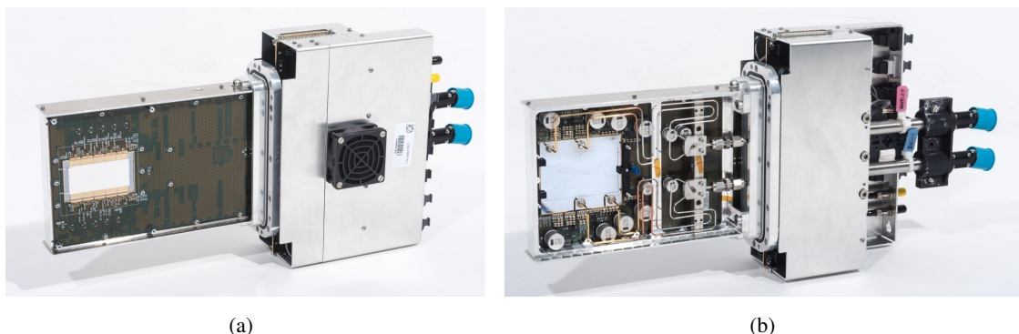
Figure 4. Photographs of a GTK station viewed from the sensor side (a) and from the cooling plate side (b).
