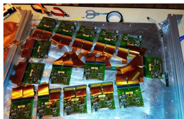
FIG. 1: Left: Detector and FEBs mounted on 10 mm Al cooling plate. Right: Schematic of experimental setup.
