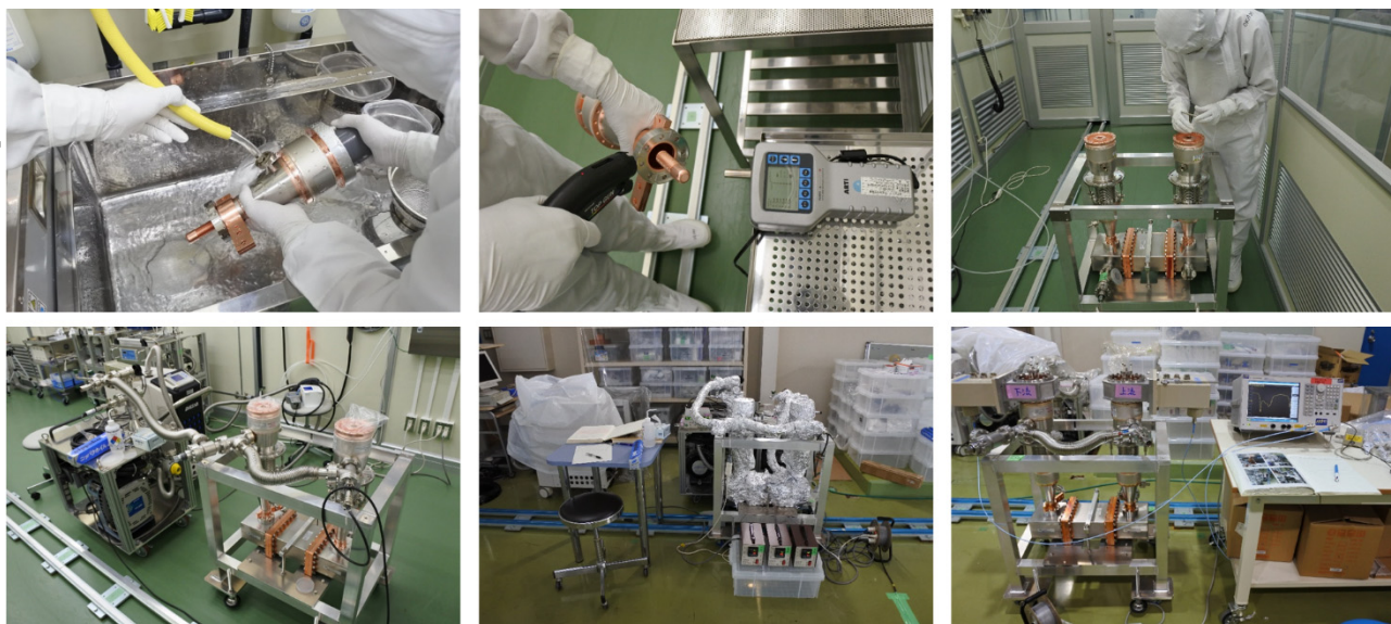
Figure 3: Status of the assembly work in the clean room, the baking, and the low power test by the network analyser. From left to right in the top figures: the ultraclean water rinsing, cleaning by the ion gun, and jointing between the warm and cold parts. From left to right in the bottom figures: the pumping and the leak check, the baking, and the low power test.
