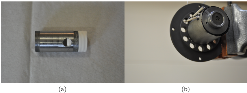
Figure 5.1: Building of the modified VADLIS with extraction plates for first off-line tests. a) Anode body mounted on BN insulator with thread. b) Connections to anode body and extraction plates.
