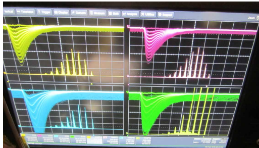
Figure 3: Waveform and photoelectron spectra of four Hamamatsu S13360 MPPCs.
