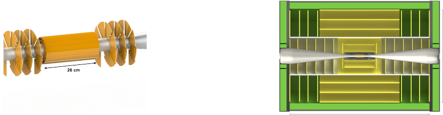
Figure 1: Layout of the CLIC vertex detector. Figure 2: Layout of the CLIC tracking detector.
