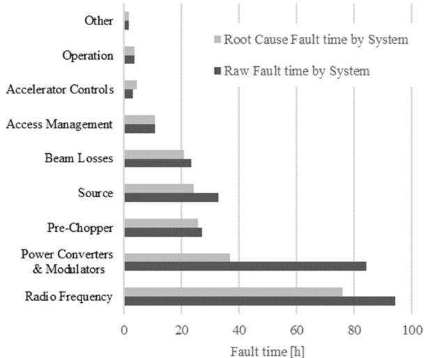
Figure 3. Linac4 systems fault times during the first two phases of the Reliability Run.
