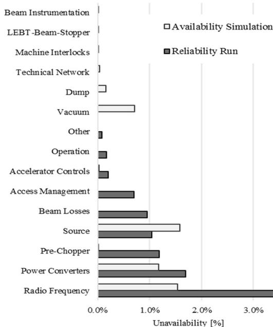
Figure 4. Linac 4 systems unavailability from Reliability Run and simulations.
