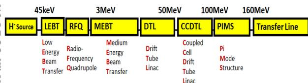
Figure 1: Linac4 basic architecture.
