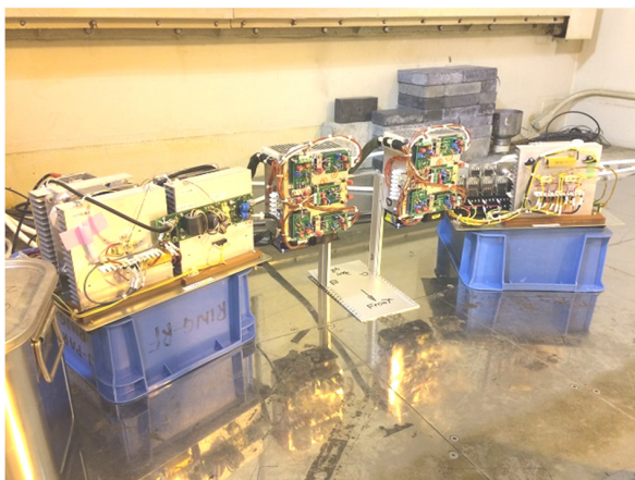
Fig. 1. The setup of irradiation test of solid state amplifier (left) at the QST. Middle and right show the setup to test MOSFETs without RF power.
