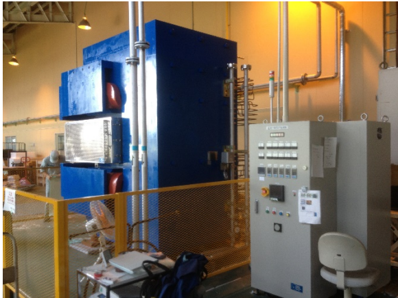
Figure 1: Magnetic annealing oven for the mass production.
