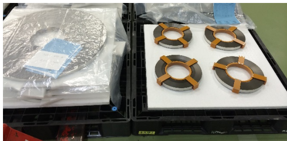
Figure 2: Magnetic alloy cores for J-PARC MR (left) and CERN PSB (right).
