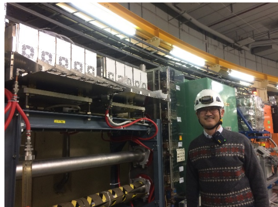
Figure 3: 10-Cell FT3L cavity for the beam test.
