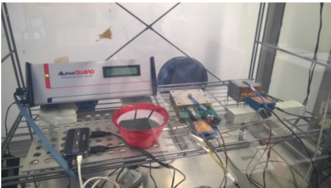
Figure 13. Measurement set-up inside the radon chamber at the Politecnico of Milano: the two RaDoM detectors, the Alphaguard reference radon monitor and the incense used to produce the particulate.
