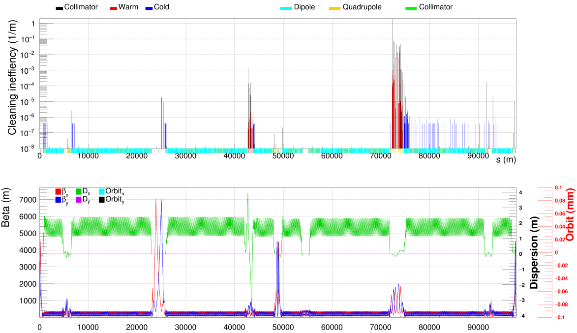
Figure 9: Image showing the full ring lossmap at injection for a horizontal beam halo.
