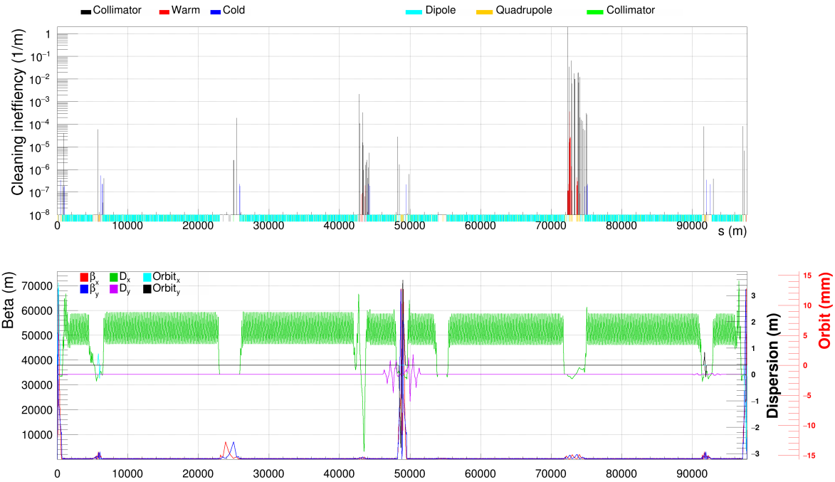
Figure 12: Image showing the full ring lossmap at collision for a horizontal beam halo.
