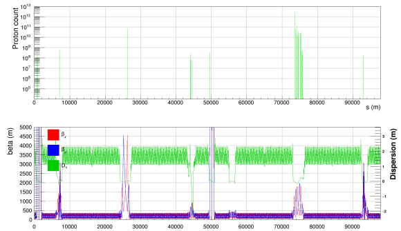
Figure 24: Image showing the loss distribution with 5 extraction kickers pre-firing.
