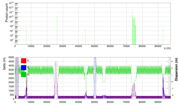
Figure 23: Image showing the loss distribution with 4 extraction kickers pre-firing.
