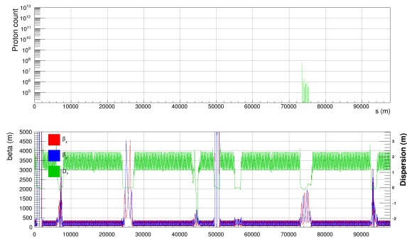
Figure 21: Image showing the loss distribution with 1 extraction kicker pre-firing.
