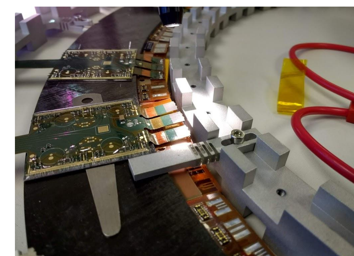
Loading tests with modules on Endcap ring local support
