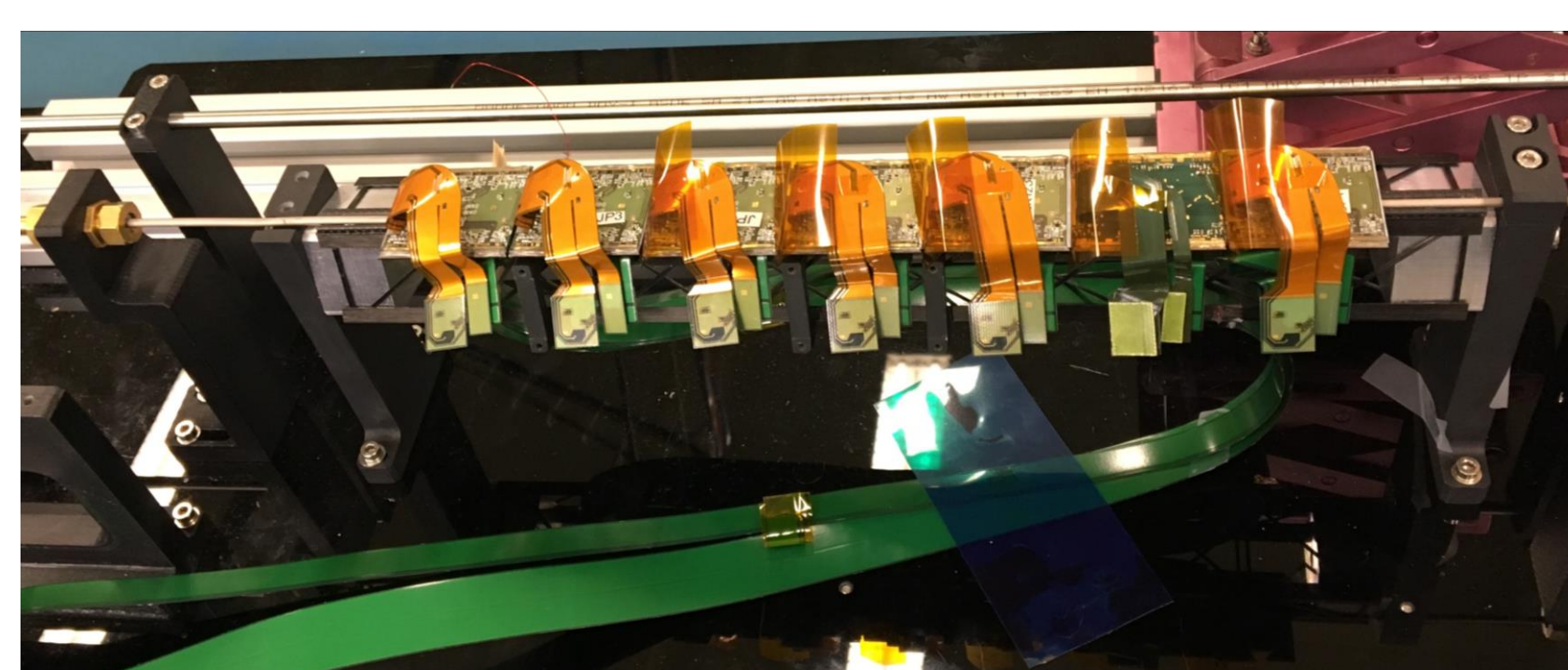
7 loaded FE-14 quad modules on outer barrel stave prototype
