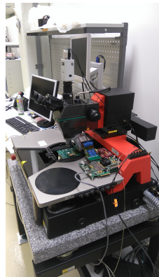
probe station for wafer test
