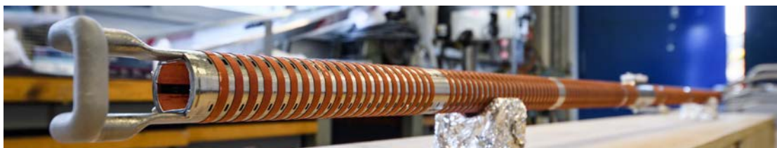
Figure 12 Finalized beam-screen prototype. Photo taken prior to shipment to ANKA
