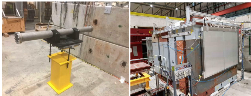
Figure 35: Replica of the SHiP target and the experimental setup as seen from behind.
