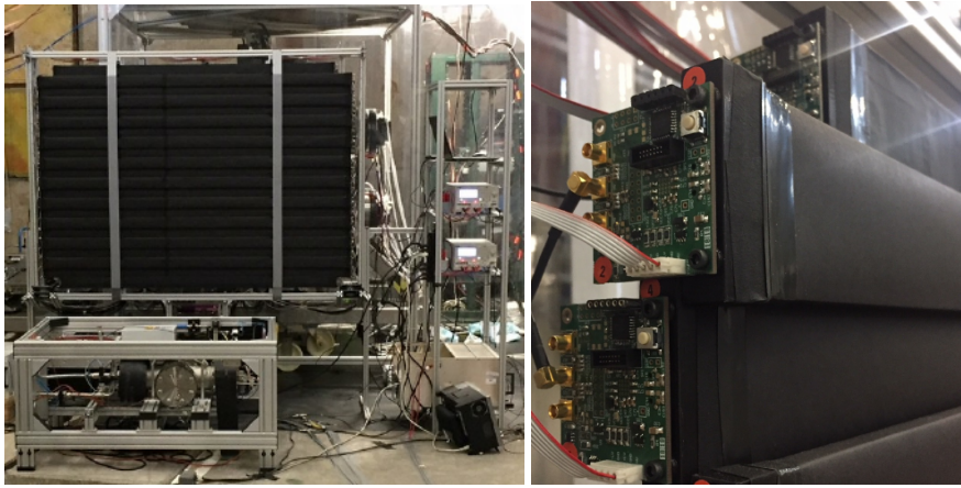
Figure 56: Left: picture of the plastic scintillator TD prototype comprising 22 bars, placed in front of a high-pressure TPC prototype and exposed to test beams at the CERN PS. Right: picture showing some of the front-end electronic boards of the TD prototype, providing a summed output signal for arrays of 8 large-area SiPMs applied to the bar surface.
