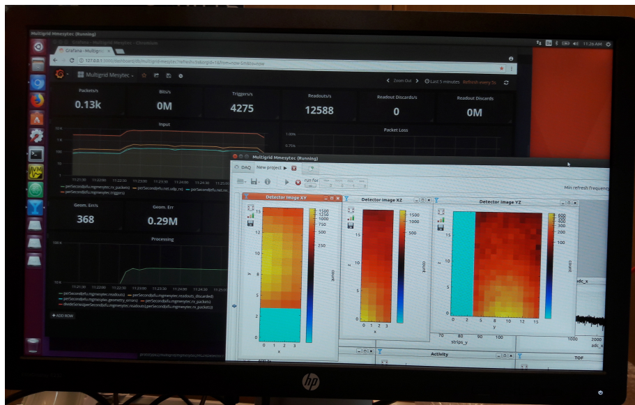
Figure 6. Grafana dashboard and live detector images from a recent test run with low neutron intensity at the Source Testing Facility at Lund University [41].
