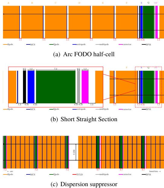
Figure 2: Layout of the arc FODO half-cell and DIS
