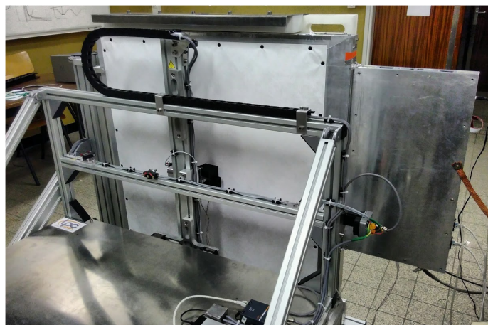
Figure 5. The Calipso quality assurance setup, which used a full scale prototype SoLid electronics enclosure. The enclosure, dubbed ‘Zoidberg’, read out over 100 million neutrons during the QA campaign to ensure a uniform plane response.
