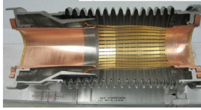
Figure 1: Example of RF fingers placed between magnet in the LHC.
