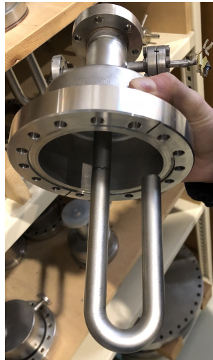
Figure 3: HOM coupler actually used in an accelerating cavity
