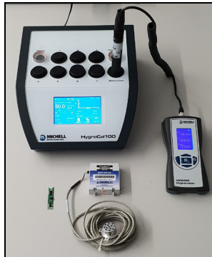
Fig. 7. Evaluation setup for humidity sensors
