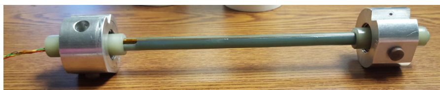
Fig. 12. PCB sensor with the G10 shaft.
