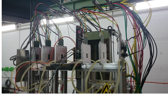
Figure 5. The DESY II test beam setup. Shown are the CCDP with the FE-I4 reference plane, together with the six planes of the telescope.
