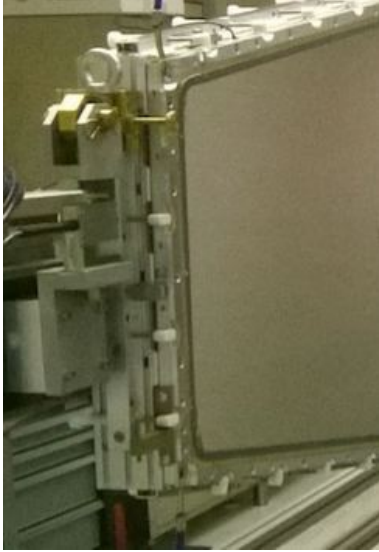
Figure 30: One of the adjustment screws for the panel alignment.
