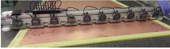
Figure 15: The limbo tool, while used to measure the planarity of a drift panel.
