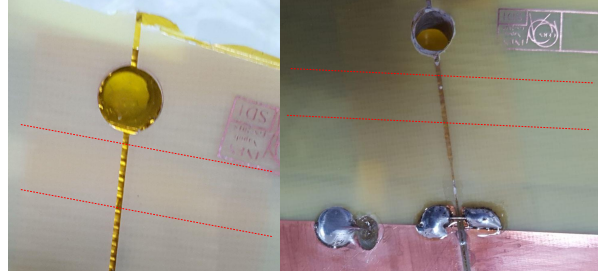
Figure 19: A junction between two PCBs in the o-ring region (red dashed lines) before (left) and after filling with Araldite 2011 (right).
