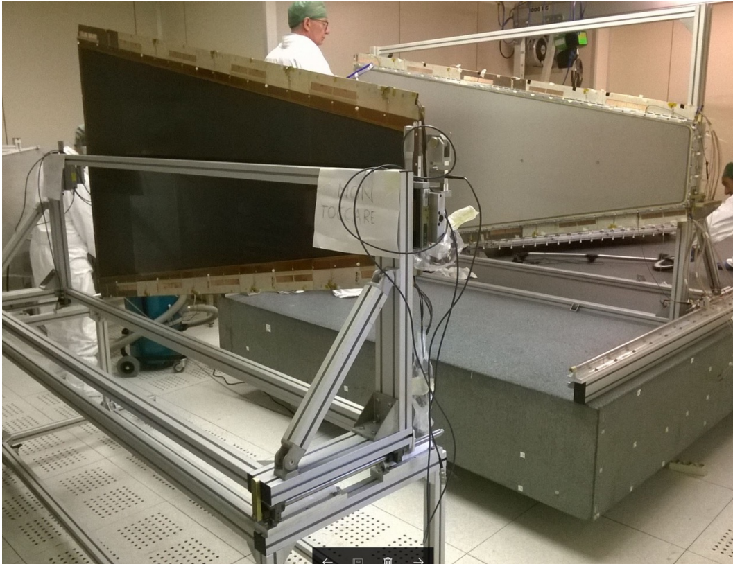
Figure 28: The granite table used for assembly, equipped with the assembly tool. The photo shows the drift panel 5 mounted on the table and the RO panel 4 ready for mounting.
