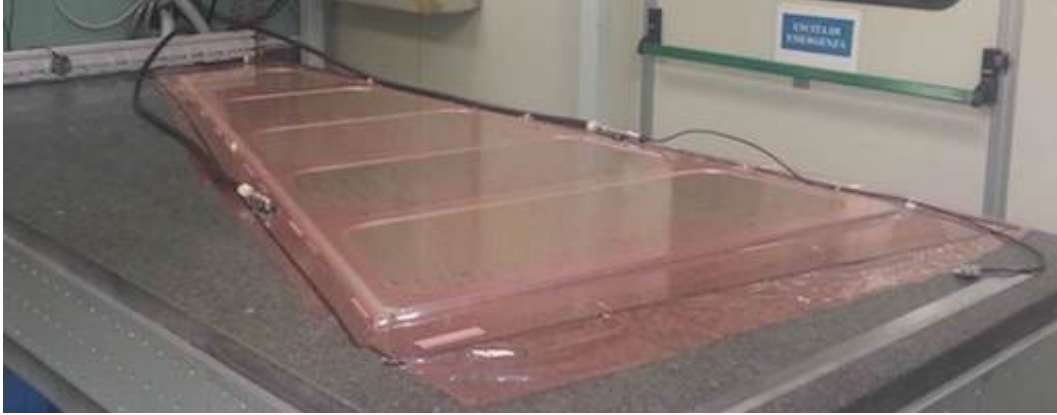
Figure 12: A drift panel during glue curing (vacuum bag technique) on the granite table.
