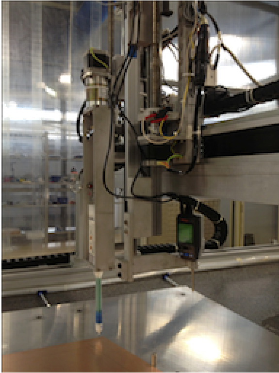
Figure 6: The height gauge of the right and the glue dispenser on the left.
