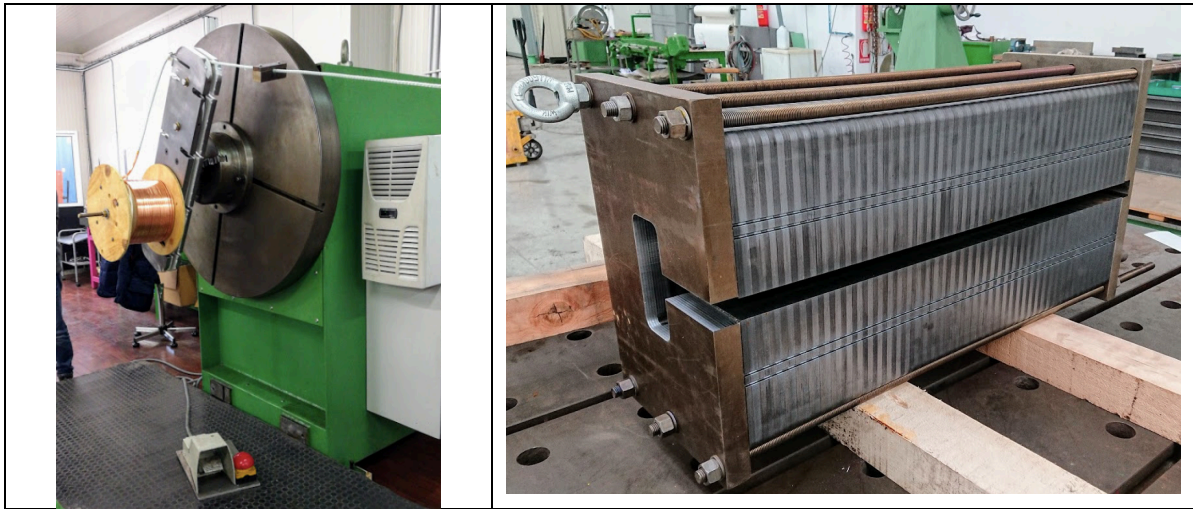
Figure 2 -The DHPTB102 dipole during different construction phases at ORMET S.r.l.
