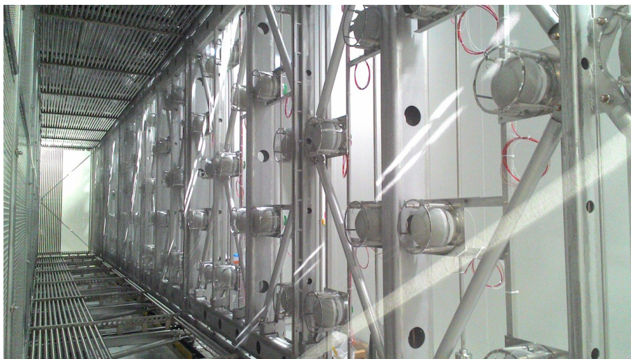
Figure 1. PMT deployment behind a TPC wire plane.
