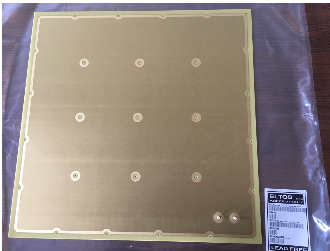
Figure 2.8: Picture of a LEM module used for ProtoDUNE-DP
