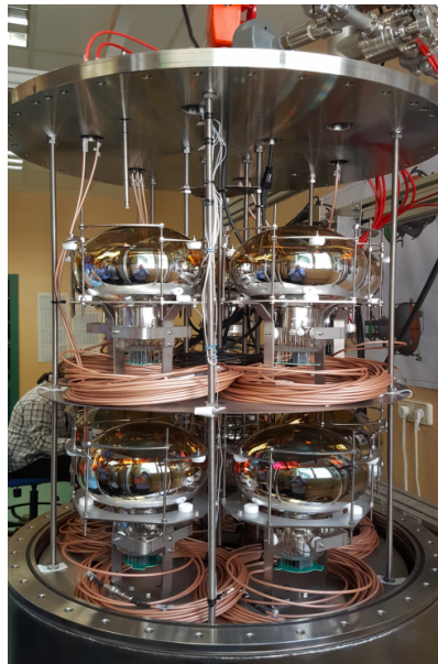
Figure 5.3: Picture of the PMTs being installed in the testing vessel used for the ProtoDUNE-DP PMTs.
