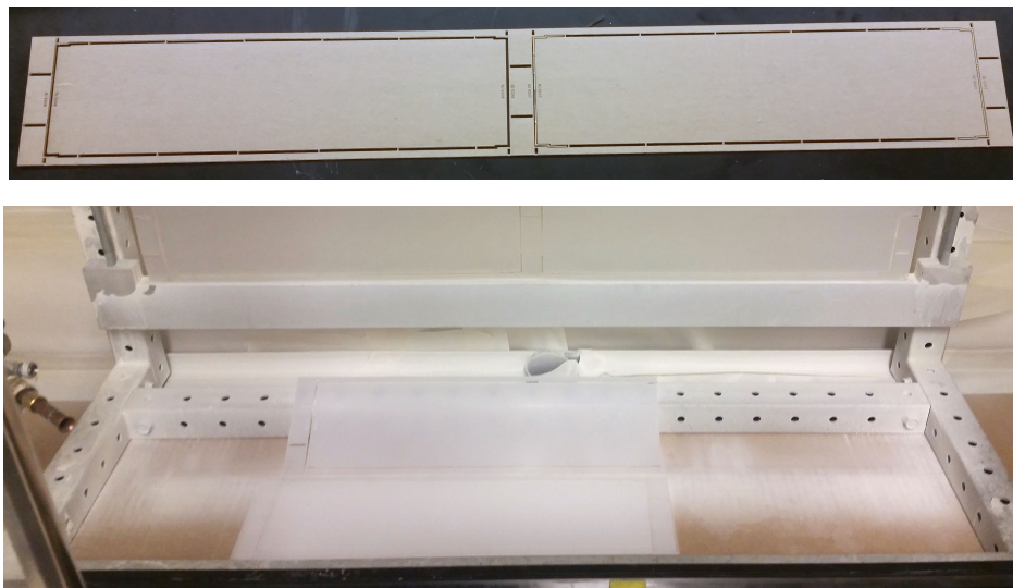
Figure 5.16: A laser-cut acrylic template holding two plates and three test tabs (top). TPB-coated acrylic plates after spraying during fabrication of parts for ProtoDUNE-SP (bottom).
