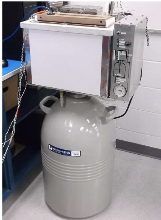
Figure 3.20: Cryogenic Test System: an insulated box is mounted on top of a commercial LN 2 dewar. Simple controls allow the box to be purged with nitrogen gas and LN 2 to be moved from the dewar to the box and back to the dewar.
