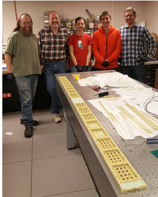
Figure 5.7: Full-scale ARAPUCA for ProtoDUNE-SP during assembly. SiPMs are visible in the sixteen cells before the installation of reflecting foils, coated filter windows, and readout cabling.
