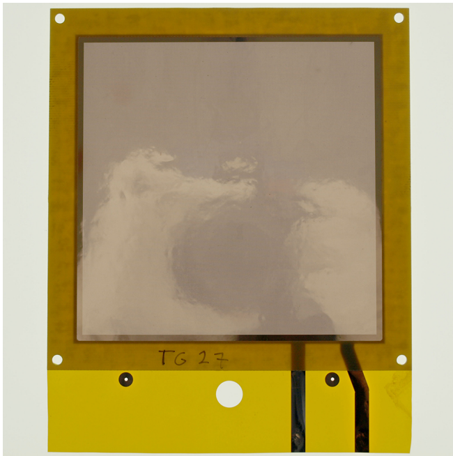
FIG. 7. The Top side of the foil. The identification of the orientation is made based on the location of the two strips seen on the lower right corner of the picture.
