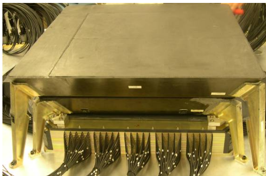
Figure 5: Refurbished CREAM calorimeter before integration of the refurbished SCD-II.
