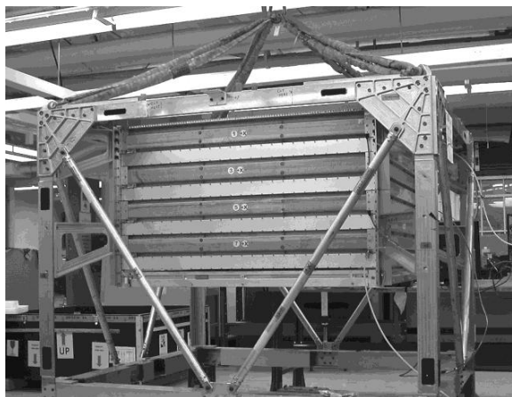
Figure 7. TRD-II mechanical pre-integration in the CREAM-VII instrument at UMD. The CD detector is also mounted.
