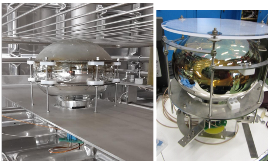
Figure 15: Left: picture of one PMT coated with TPB. Right: a PMT unit with the coated plate mounted in front of the photo-cathode and ready for its installation.
