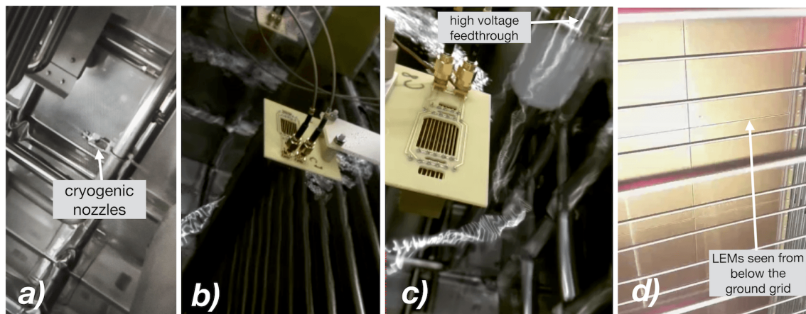
Figure 20. Images of inside the cryostat provided by the four cryogenic cameras. Camera a) monitors the functioning of the cryogenic nozzles during cool down. The liquid level during operation can clearly be seen by cameras b) and c). Camera d) is placed under the ground grid and cathode (clearly visible on the picture) and observes the 50 \times 50 \text{ cm}^2 LEMs.
