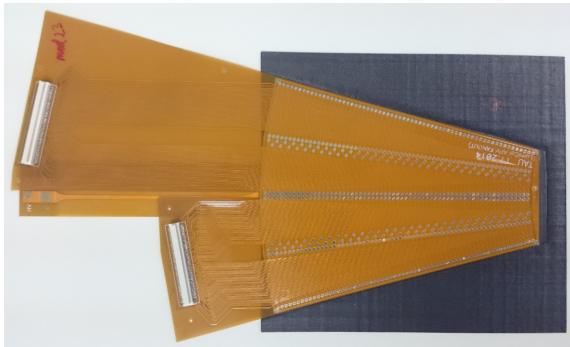
Figure 9: A thin LumiCal module. The black part is the carbon fiber support. The silicon sensor is covered by the Kapton-copper fan-out which has two connectors for front-end boards.
