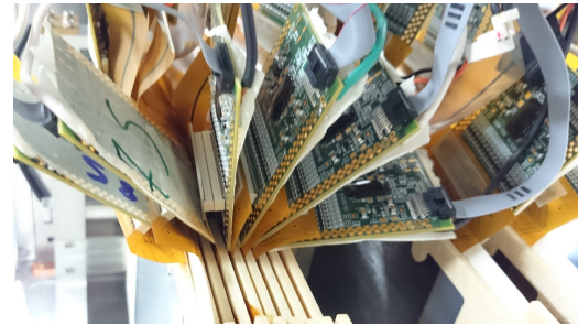
Figure 12: An APV25 hybrid front-end board connected to LumiCal modules.
