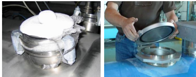
Figure 5. The original DN90-mm spring-loaded relief disk after the 2008 accident (left) and the newly developed DN200-mm (right) plate disks for the up-graded protection of the LHC cryostats.
