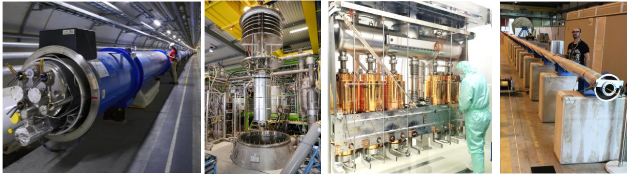
Figure 1. Some examples of helium cryostats for accelerator devices at CERN: (from left to right): the LHC dipoles, the HFM vertical test cryostat, the HIE Isolde cryo-module (before insertion in its cryostat), a 60-m prototype of a SC link for HL LHC.
