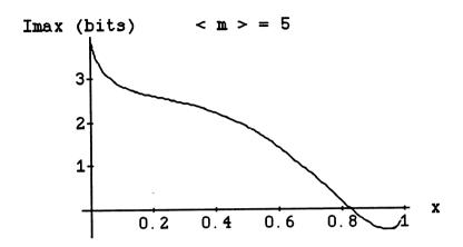
Figure 1: Here we plotted the maximum amount of information (in bits) that could be conveyed by pulses with a mean number of five photons. Observe that  $I_{\text{max}}$  decreases very fast with increasing x. Unfortunately, owing to our approximation, an unphysical negative tail develops at  $x \approx 0.8$ .
