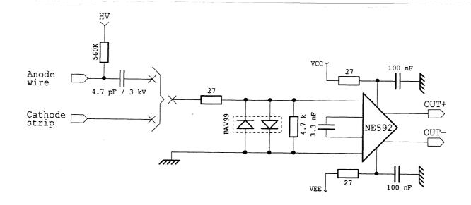
Fig. 3 Preamplifier circuit diagram
