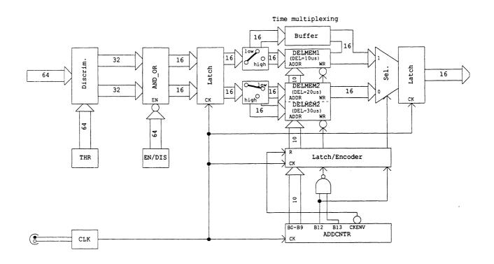
Fig. 4 The ADMUX2 block diagram
