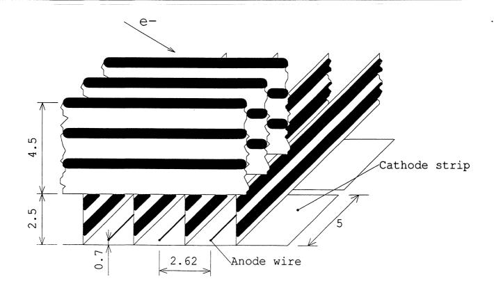
Fig. 1 Detail of the MWPC
