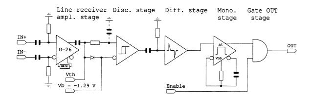
Fig. 5 Discriminator block diagram
