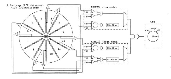
Fig. 2 Readout system block diagram
